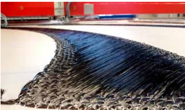
Large TFP parts made with fast fibre laying
