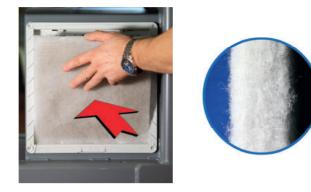
Inserting filter element Filter element cross section (compacted side left)
